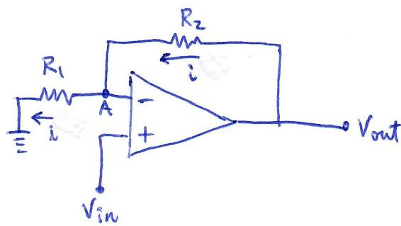
ideal opamp: \* voltage input equal:  $V_{in} = V_A$ .
