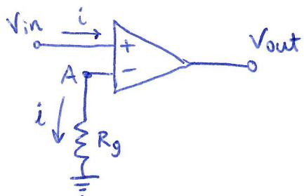
$$\left. \begin{array}{l} V_{out} = K(V_{in} - V_A) \\ V_A = iR_g, \quad V_{in} - V_A = iR_{in} \end{array} \right\}$$
