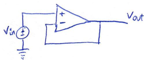
$$\text{we have } V_{out} = K(V_{in} - V_{out}) \Rightarrow V_{out} = \frac{K}{1+K} V_{in}$$
